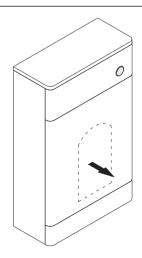
Remove the front panel from the unit and cut the hole to allow the waste pipe and flush pipe to pass from the cistern
