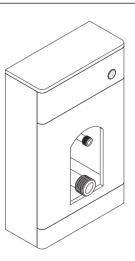
It is recommended to seal the cut edge and bottom edge of the unit, to protect against moisture ingress
