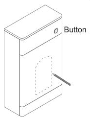
Mark these dimensions on to the front panel of the unit using a pencil
