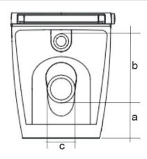
Measure the height from the floor to height a then measure height b and allow 5mm tolerance, then measure width c and allow 5mm The flush button can be installed on either the left/right side
